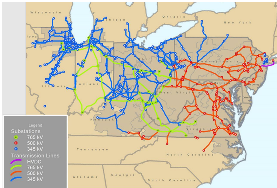
Figure 17. PJM’s backbone transmission system 27
